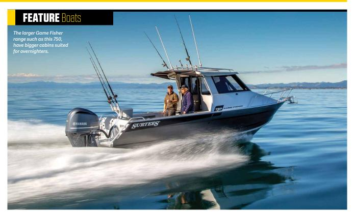
A key reason the boats are popular is their non-pounding deep V hull design. This provides a comfortable ride for all on board with its very fine-entry point, variable from 15 – 20 degrees deadrise at the stern depending on the length of the hull. This allows you to cut through choppy water. Typically, a deeper V hull design usually means a trade off in stability while at rest, not with Surtees as our Anti-Roll Stablishing Ballast Technology ensures you have a stable and safe boat.
