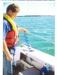
above: Wash down hose: Is an excellent optional extra. Note the vinyl covered seat that is clipped onto the wide side shelves and the small round deck light.
