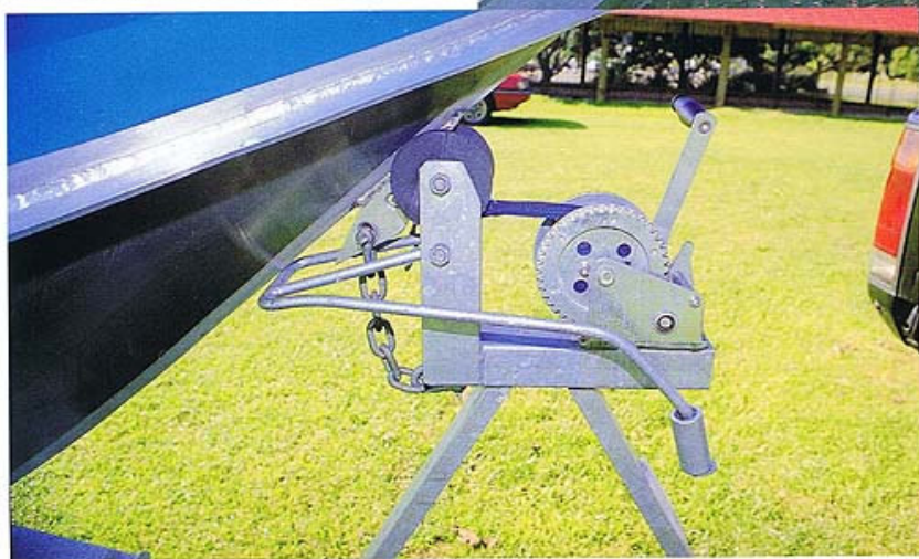
A cleverly designed trailer catch allows drive-on, drive-off boating
