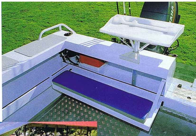
The transom face folds down to form a stern seat.
