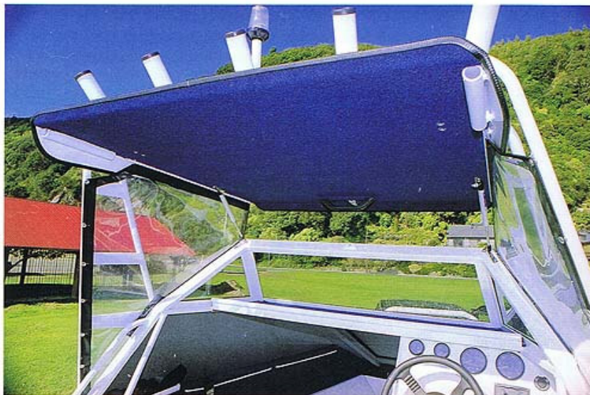
With the hardtop in "up" position a space opens above the 'screen' for improved ventilation and vision.
