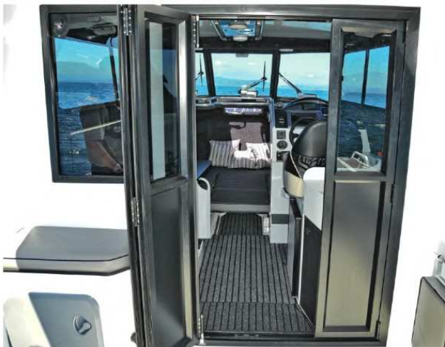
Above: Folding doors and a window that drops vertically into the bulkhead provide ventilation and communication with the cockpit, while still allowing security and shelter when closed. Right: The port-side of the cabin has bench seats and an adjustable table that can be reconfigured into a berth.
