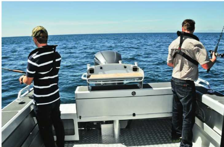
The spacious cockpit provides top-of-the-thigh support for anglers; a transom battery locker/bench seat, transom step-through and bait station are other features.
