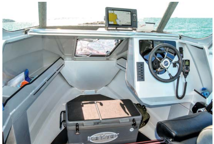
Access for the bowman is through a large forward hatch with a platform to stand on in the fore-cabin.
