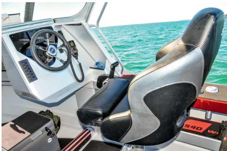
Helm seating is provided by a nicely upholstered sliding, swivelling, bucket seat with roll-back bolster and gas-shock pedestal.
